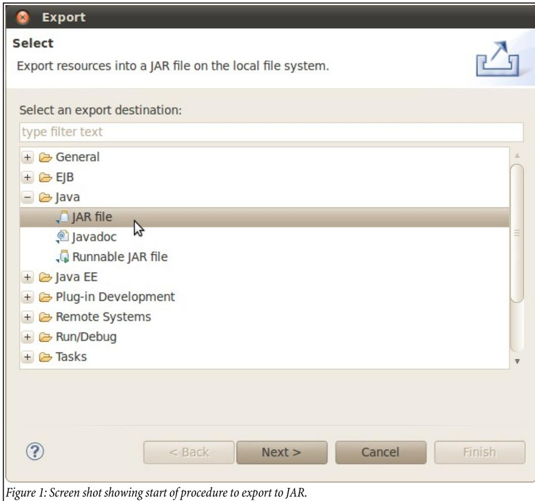
Figure 1: Screen shot showing start of procedure to export to JAR.
